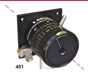
The continuously variable attenuator precisely controls power **and** polarization of a transmitted  $\mathrm{CO}_2$  laser beam. The other beam parameters such as alignment stay unaffected. The instrument contains two rotatable grid polarizers in a compact housing. It can be used alone or directly mounted on a  $\mathrm{CO}_2$  laser.
