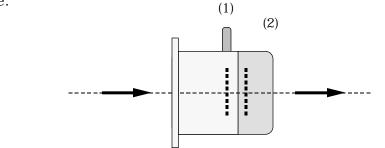
Four mounting holes 3.2 mm in diameter at a spacing of 40 mm are provided in the flange. The attenuator/polarizer functions do not depend on the angular alignment within the clear aperture. Due to a slight inclination of the elements no reflected light can leave the housing.
