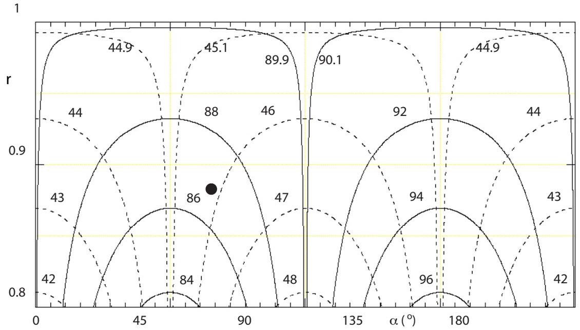
As an example we use the measured recording shown above in section 10.B. The result is represented as a black dot in the tuning graph. From this graph it becomes clear that  $\alpha_0 \approx 45.8^\circ$ ,  $\delta \approx 86.8^\circ$ ; this uniquely determines how to adjust the phase retarder mirror in order to achieve perfect circularity ( $r=1$ ).
