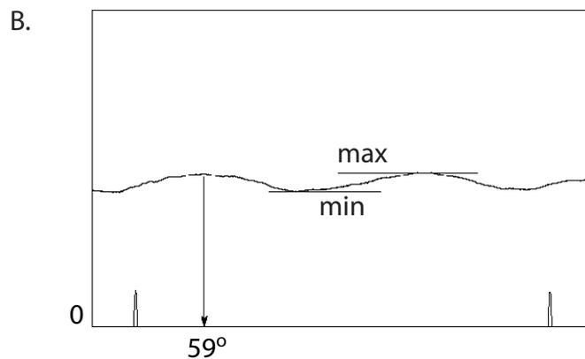
This situation is typical for the machining application with a circularly polarized CO<sub>2</sub> laser beam. The polarization here is not perfectly circular because the power remains modulated, with a power ratio  $r = P_{\min}/P_{\max} \approx 0.88$ . The maximum power signal is seen to occur at an angular position of  $\alpha \approx 59^\circ$  from the encoder peak, i.e. from the vertical, in anticlockwise direction as viewed from the laser.
