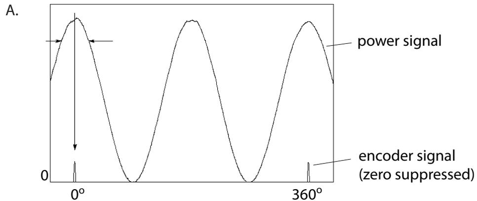
This is an example of a linearly polarized laser beam with vertical field orientation, since the power is modulated down to zero at the times of horizontal orientation of the polarizer (90°, 270°).
